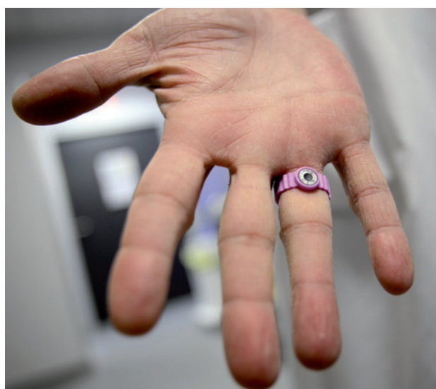
Dosimetric finger ring used by the nuclear medicine unit personnel in the North Saint-Denis Cardiology Centre
