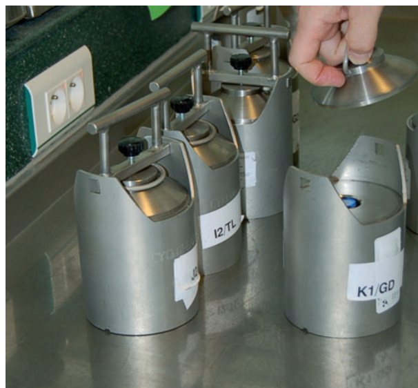
Packaging of sealed sources, nuclear medicine unit of the Nancy university hospital
