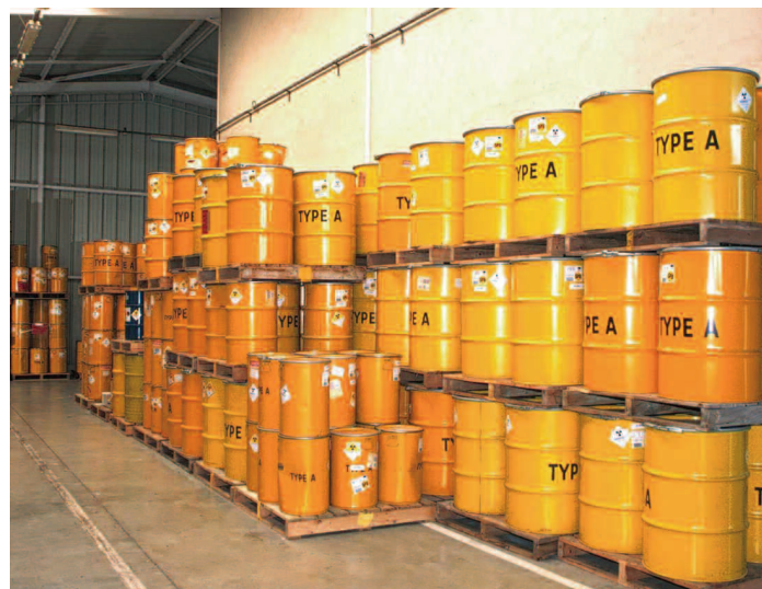
Metal drums containing low level waste stored at CEA in Saclay (Essonne département )
