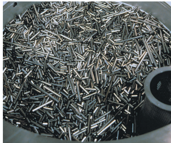
Fuel assembly hulls, ACC facility – AREVA NC at La Hague (Manche département)
