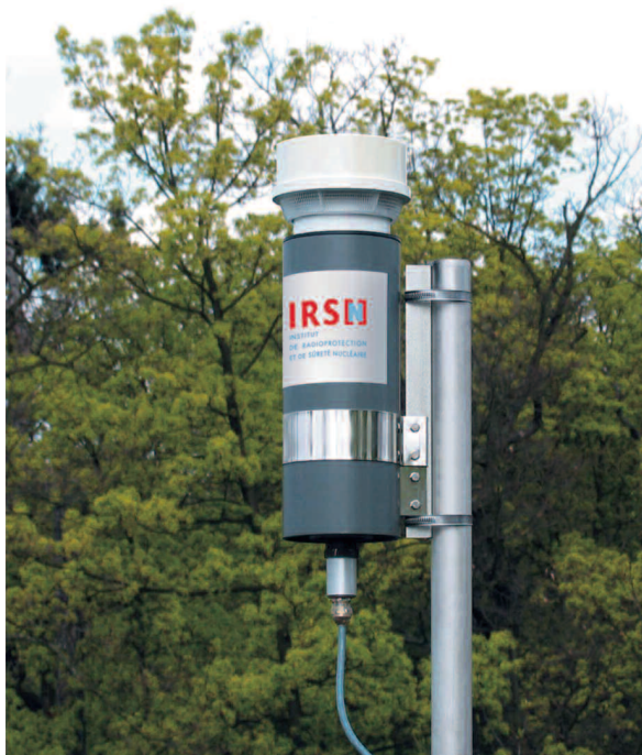
Téléray surveillance network: monitor continuously measuring ambient gamma radioactivity in the air
