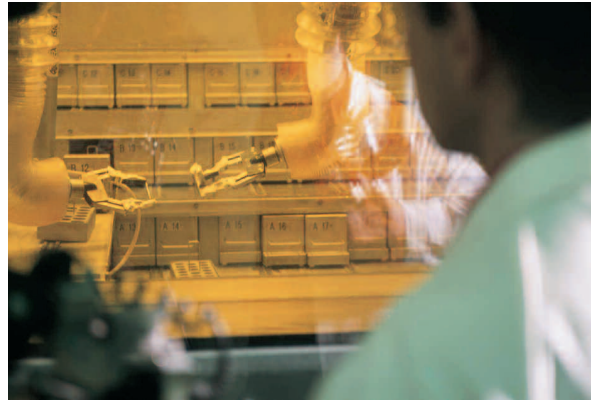
Operator remote-handling radioactive materials in one of the LECI cells in Saclay (Essonne département )
