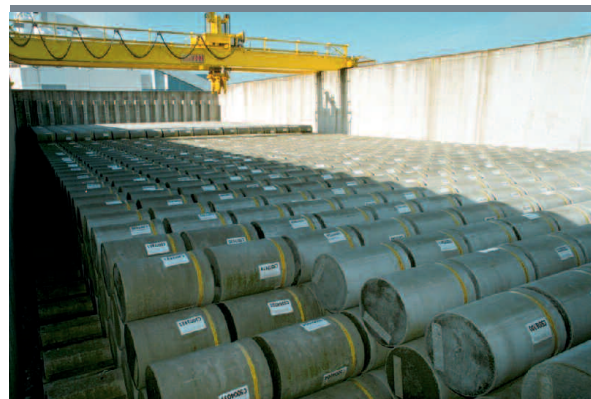
Storage of waste drums in the ADT facility – AREVA NC at La Hague (Manche département)
