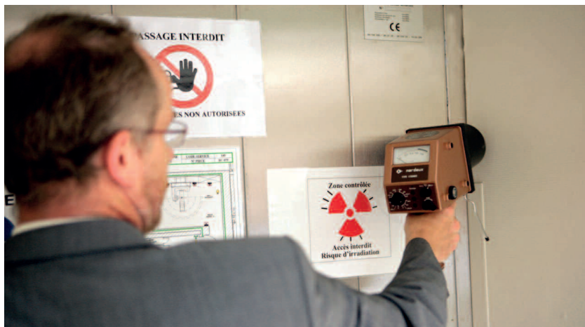
Dose rate check using a babyline at the CHU Henri Mondor University hospital in Créteil – August 2008
