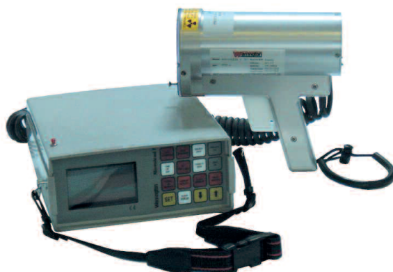
Portable X-ray fluorescence device to locate lead in paint – ARELCO
