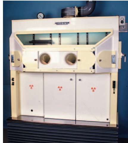
Shielded chamber for handling unsealed radioactive sources used in nuclear medicine
