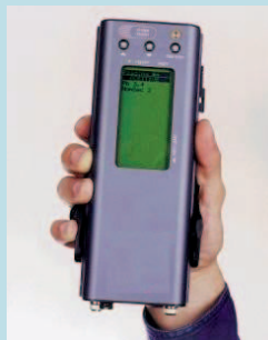
Portable X-ray fluorescence appliance for detecting lead in paint
