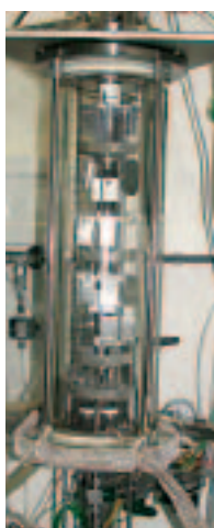
Autoclave used for experiments to qualify the chemical cleaning process
