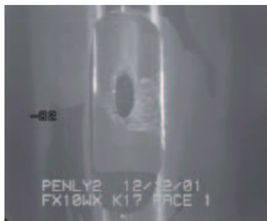
Fuel rod perforation due to vibratory wear at bottom grid assembly level
