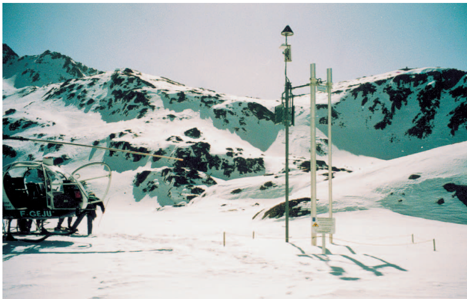
Snow height measuring device equipped with a caesium 137 source
