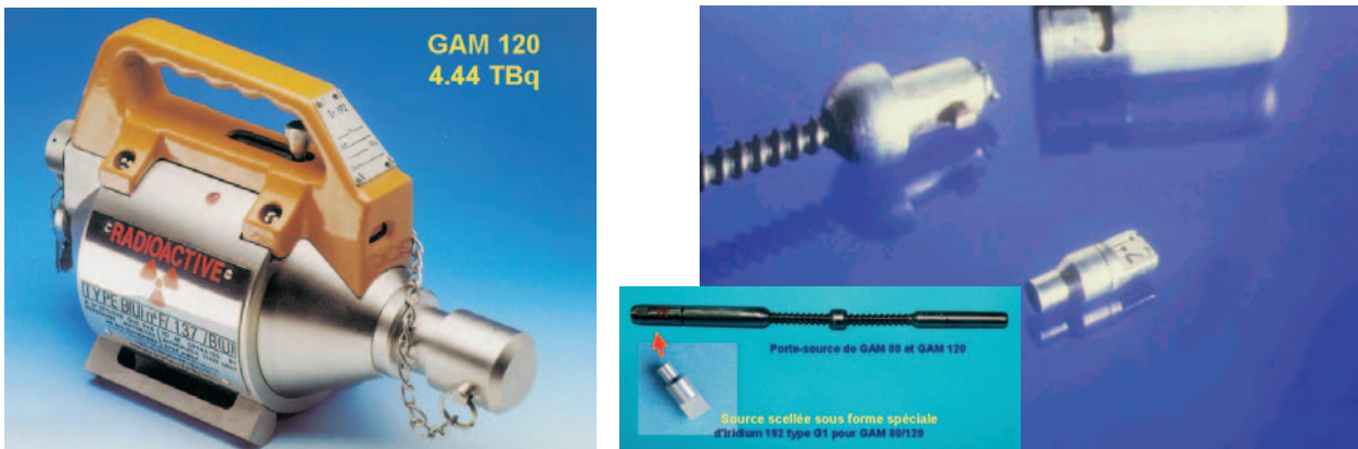
Gamma radiography device and its radioactive source
