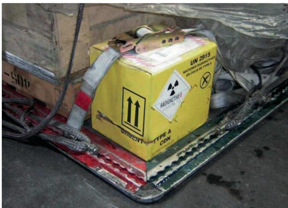
Photo of a package damaged by a fork-lift truck
