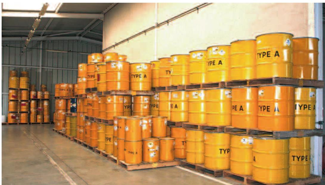
**Interim storage of low-level waste packaged in metal drums pending reprocessing (CEA/Saclay)**
