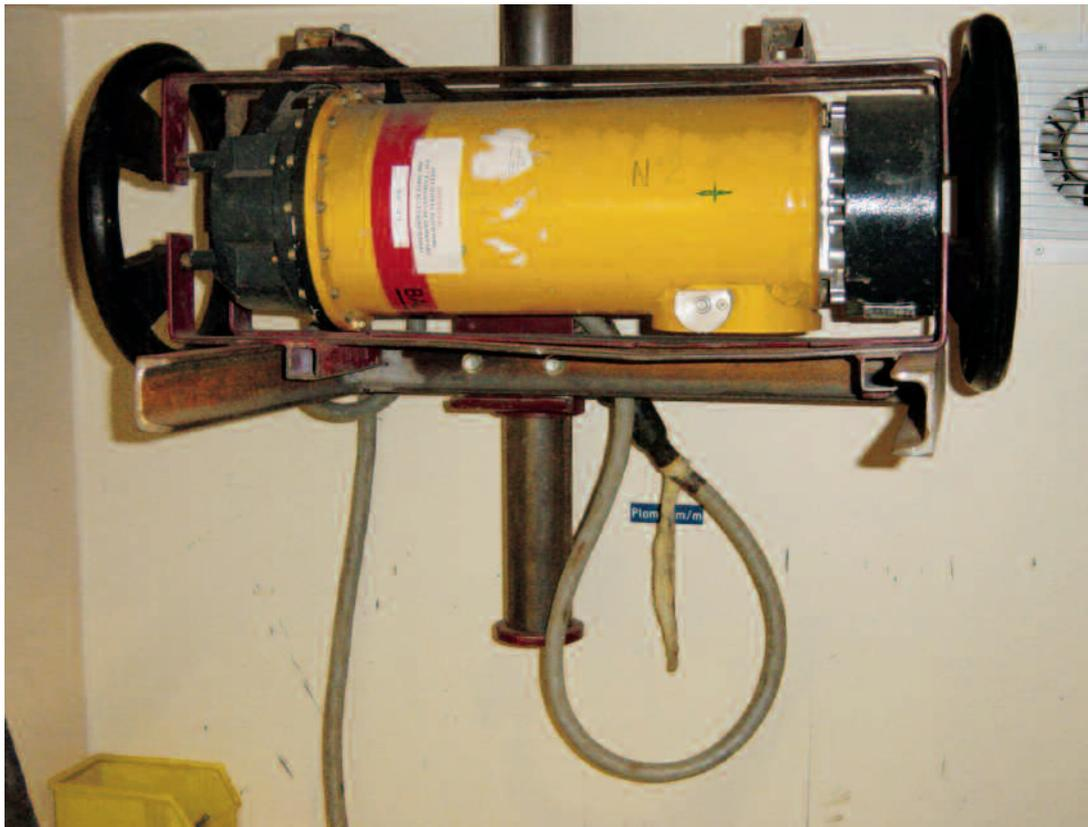
Electric X-ray generator in a radiography chamber
